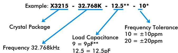
This part number example given will provide a 32.768kHz crystal in X3215 package with  $\pm 10$ ppm calibration tolerance at 25°C and a load capacitance of 12.5pF.
